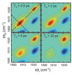
**Fig. 3.** 2D-IR spectra of free HRP as a function of increasing  $T_{\rm w}$ . The dashed lines illustrate the diagonal and antidiagonal slices through the data for calculating the eccentricity parameter.
