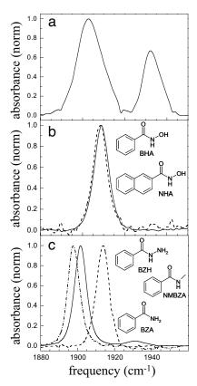
Fig. 1. Normalized FTIR spectra of the CO-stretching mode bound to HRP in the free form (a) and when complexed to 2-NHA (dashed line) and BHA (solid line) (b) and NMBZA (dash-dot line), BZH (dashed line), and BZA (solid line) (c). Structures and abbreviations of the substrates used in this study are shown in the appropriate places.
